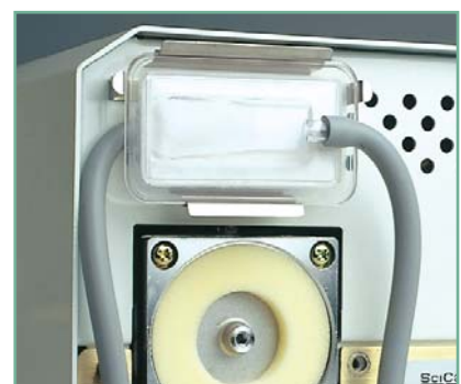
An important biological filter will not allow bacteria or spores above 0.3 \mu m to enter the sterilising chamber during the drying cycle. An efficient air filtration system includes easy access filters for quick replacement
